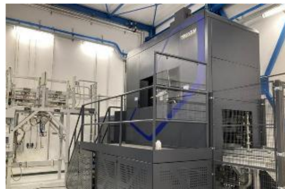
Nikon SLM NXG XII 600 4 lasers - Zone fabrication 600x600x600mm
